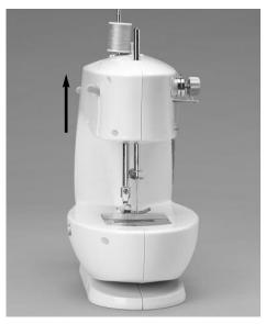
Lift the presser foot and place fabric under the presser foot.
